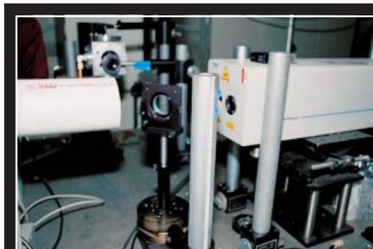
Experimental setup showing the target chamber and the LIBS laser
