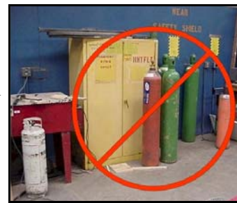
Unsecured & uncapped cylinders safety hazards
